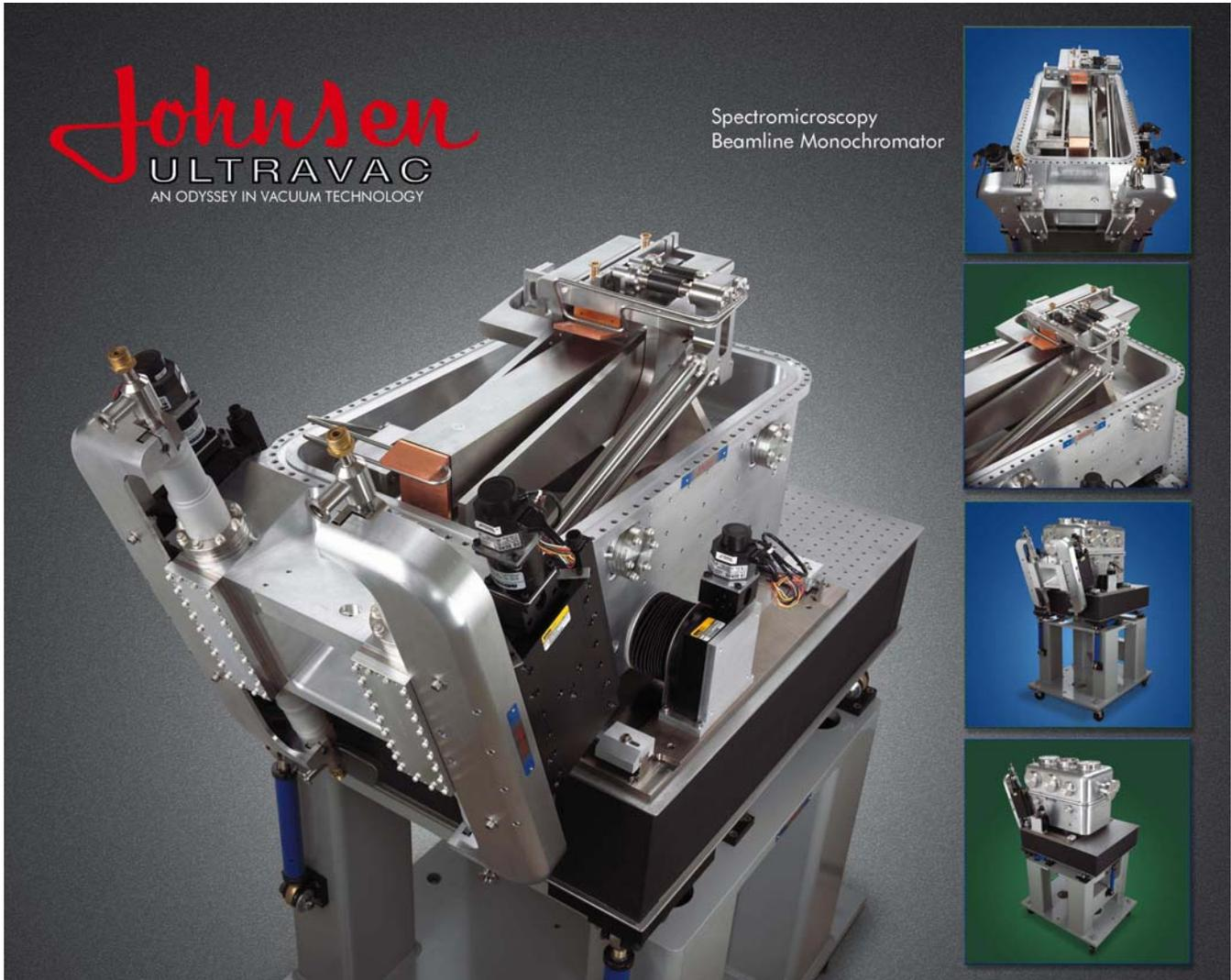
Production stage photo of JUV Monochromator (shown with lid removed and installed dummy optics).
