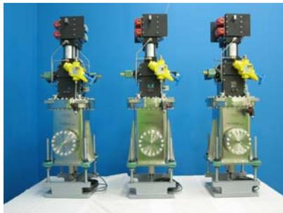
2. The overall shutter block provides sufficient thermal protection: The photon shutter blocks are designed and fabricated for a minimum of 1.15KW of heat energy incident upon either shutter block applied over an area of 25mm x 25mm centered vertically and horizontally on the shutter block face with a maximum heat density of 2.7W/mm<sup>2</sup>.
